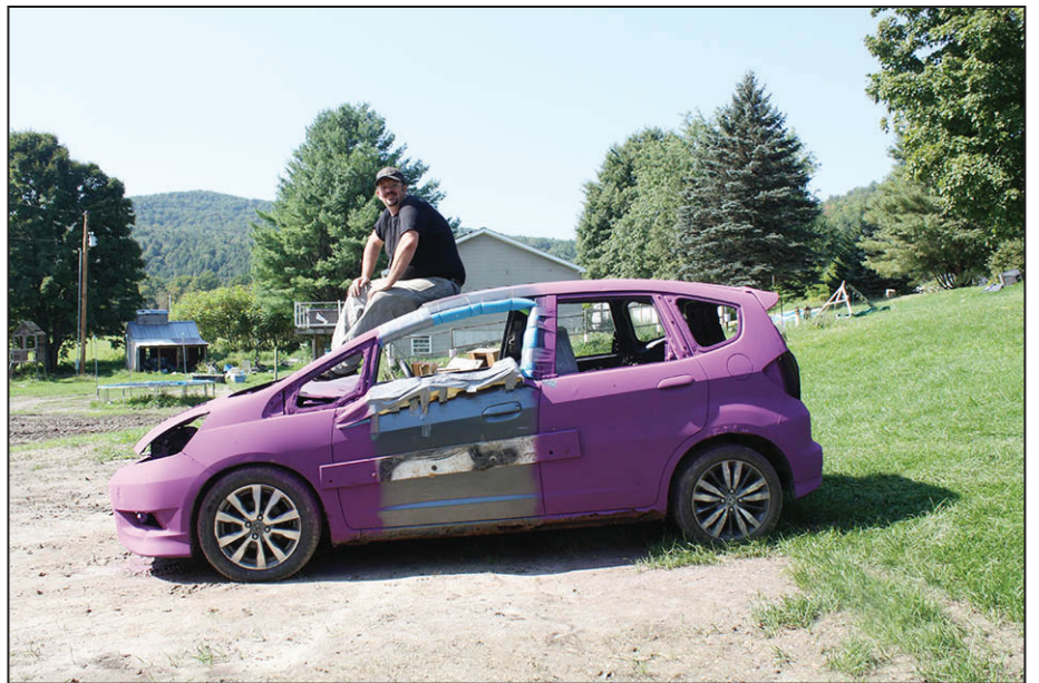
Frank Flemings Jr. shows his stripped-down car, outfitted for the Double Figure 8 races at the Champlain Valley Fair. The door has been reinforced with a piece of a blade from the old town grader and foam rubber pool noodles provide extra cushioning around the frame of the driver's door. Flemings is ready to paint the number and sponsor's name on the car and it will then be ready for its ride out of Huntington on a flatbed. See article beginning on page 12. Photo: Heidi Racht
