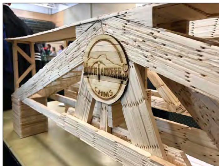
Camels Hump Middle School Engineering Club members competed in the Vermont State Bridge Building competition at Vermont Technical College in Randolph, creating a bridge one meter in length and holding almost 800 lbs. made with popsicle sticks and glue. Courtesy photos
